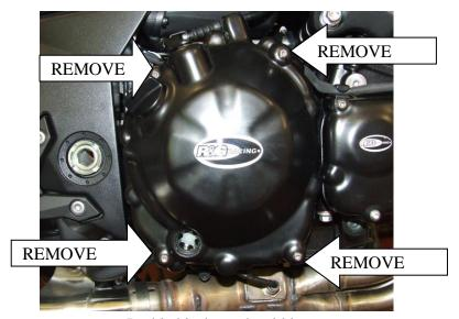
In this kit there should be: 1 x Engine Case Cover (ECC0076) 4 x M6x40mm CAP HEAD BOLTS
