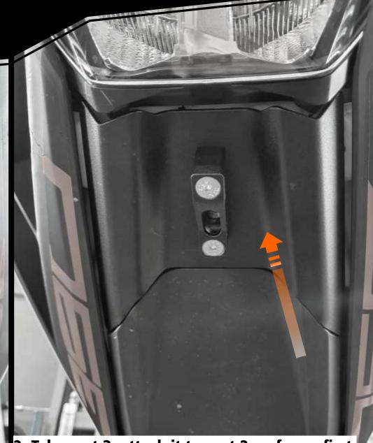
2. Take part 3, attach it to part 2 on frame first and attach part 5 with bolts B1 and B2.
