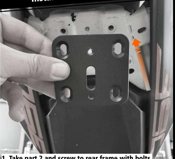
1. Take part 2 and screw to rear frame with bolts E. Fully tighten.
